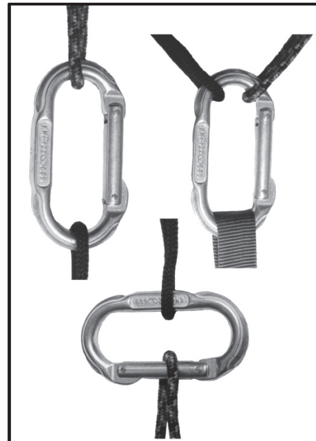
Figure 3-12. Major and minor axes and three-way loading.
