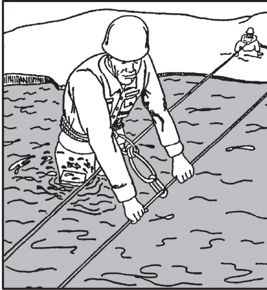
Figure 9-4. Stream crossing using a handline.
